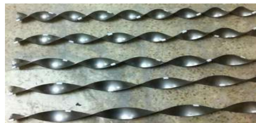
Figure 4. Aluminium Twisted Tape (Enlarged view)
