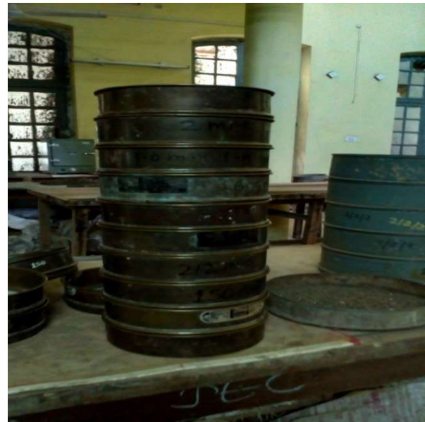
Figure 1. Set of Sieve in Lab.
