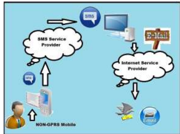
Figure 1: Working System of SMS Process Via Non GPRS Mobile
