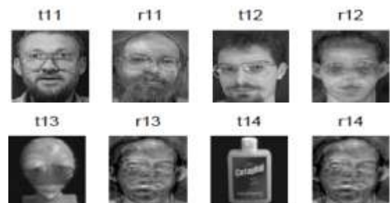
Figure-5:- Unknown face and Non-face images - t11 and t12 are unknown faces. t13 and t14 are non-faces. r** means the reconstructed image
