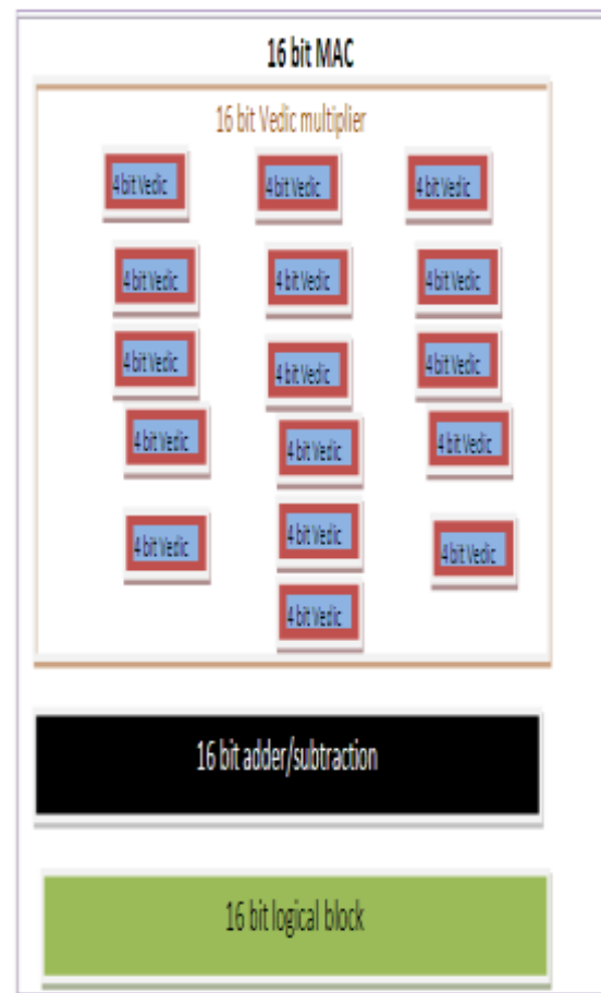
Figure 3- 16 bit Vedic MAC (Multiply and accumulate)
