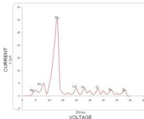
Figure 1: Direct Pulse Polarogram
